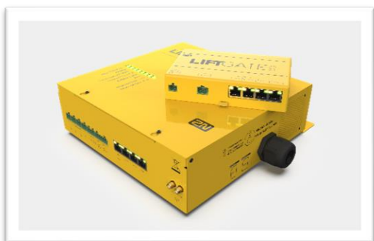
2N LiftGate IP- Gateway
